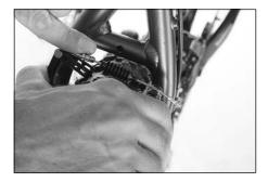
Insert the cable in the yoke.
