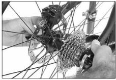
Disk brakes: Insert the wheel so that the brake disk can be easily pushed between the brake pads.
