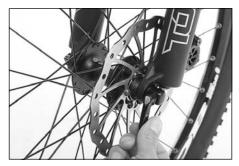
Turn the nut counter-clockwise until the wheel can be removed from the frame or front forks without any great effort. Should the nut come right off the screw please ensure that the little springs do not get lost.
