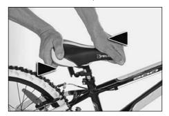
Try to move the saddle in its clamp with alternate up and down movements. It should not be possible to move the saddle.
