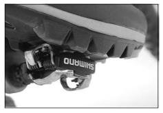
The shoe is now firmly vertically connected with the pedal. Depending on the pedal system the shoe has sidewards freedom of movement.
