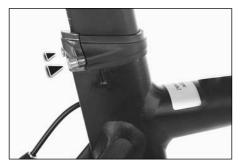
For clamping without a quick release a hexagon socket and a torque wrench of the appropriate size are required. Please also consult your dealer.
