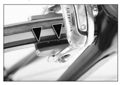
Check centring of the brake shoes. The brake shoes must be equidistant from the rim on both sides. 6.8.2 Check rim brakes and cable (mountain bike version).
