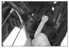
Swivel the Locking Lever so that the brake is fixed in place again.
