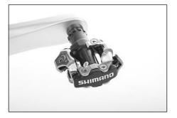
With click-in pedals the shoe and pedal are firmly connected in a vertical direction. When pedalling you can not only push the pedal down but also pull it upwards. To be able to used a click-in pedal to the full you need shoes specially designed for the pedal system concerned and to which the pedal hooks supplied with the pedal can be affixed.
