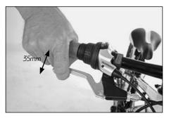
Try to push the bike with the brakes applied in this way. Both wheels must remain Locked.
