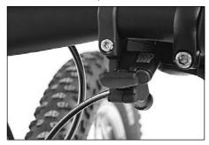
If your forks have a fixed adjustment mechanism as shown in the illustration, please read its instructions in the suspension fork manufacturer's component instructions. Suspension forks with elastomers and/or steel springs are only suitable for one overall weight range (= weight of rider + any luggage). This weight range is usually within 10 kg.
