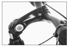
Many bikes are fitted with an adjustable stem, the height and angle of which can be adjusted. Only have adjustment carried out in a specialist workshop!
