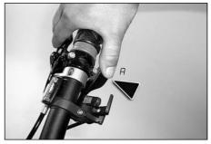
For rapid shifting through several sprockets press the Lever right down and keep it depressed until the desired gear is selected.
