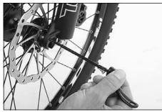
Place the springs and the nuts on the bolt. Turn the right end now protruding from the hub and the nut clockwise.
