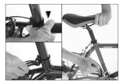
2. Withdraw the saddle with seat post from the frame.
