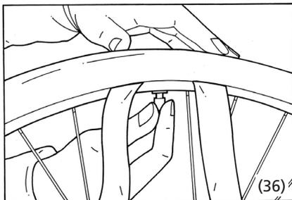
9. Return the tyre to its original position with your hands. It is very easy to cause a puncture with the tyre levers. Work from the valve holder and ensure that the inner tube does not become jammed between the rim and the tyre.
