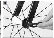
When continuing to close the lever the resistance you feel should increase significantly and towards the end even more strength is required to close the lever. Use the ball of your thumb while your fingers pull on an immovable part, such as the fork (d) or a rear stay, but not on a brake disc or spoke, to push it in all the wav.
