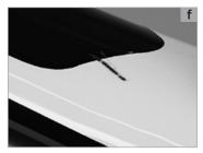
Deformed components, especially components made of aluminium, can break without previous warning. They must not be repaired, i.e. straightened, as this will not reduce the imminent risk of breakage. This applies in particular to the fork, the handlebars, the stem, the cranks, the seat post and the pedals. When in doubt, it is for your safety always the better choice to have these parts replaced. Ask your SCOTT dealer for advice.
