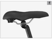
If the saddle rails fit into the clamp grooves, slide the saddle on the seat post and ensure that the clamp is positioned midway along the total length of the rails (a). Position the saddle so that its upper surface is parallel to the ground. Tighten the bolt gradually and make sure
