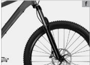
Damping is usually done by oil. To work perfectly, the fork has to be adjusted to the weight of the rider, the sitting posture and the intended use (a). Be sure to have this adjustment carried out by your SCOTT dealer at the time of delivery. For more information see the chapter "Front suspension" in your detailed SCOTT owner's manual as well as in the manuals of the suspension fork manufacturer on the enclosed SCOTT info CD.
