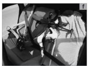
Do not combine carbon handlebars with bar ends or an aero bar, unless they are specifically approved. Do not shorten carbon handlebars or clamp the brake levers and shifters more in the middle than indicated or needed. Risk of breakage!
