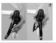
**SRAM** brake levers/shifters (a) have only one shifter that is located behind the brake lever. With one complete sweep of the shifter, the rear derailleur shifts in a higher gear by one to two chainrings or three sprockets. With a short sweep the chain changes to the next smaller chainring or sprocket.
