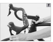
To check whether the headset runs smoothly, lift the frame up until the front wheel no longer touches the ground. The handlebars should turn from far left to far right without feeling roughness or tightness at any point. With a gentle tap on the handlebars the fork should turn easily from the middle position (a).
