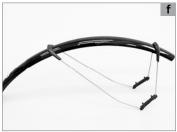
For safety reasons the front wheel stays must have security fastenings. They prevent the tyre from being blocked by impurities taken up by the front wheel from the ground. In this case the security fastening frees the stay and hereby prevents a possible accident. The plug connection can easily be refastened.
